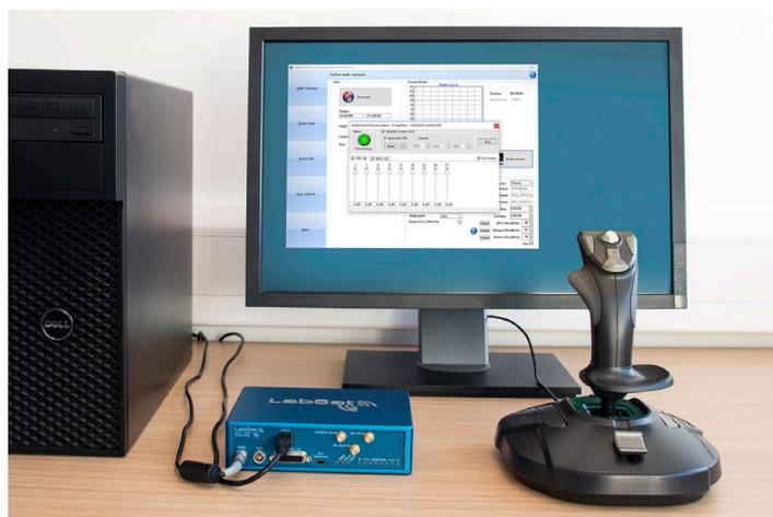
LabSat RT can play satellite signals from two constellations with a current time stamp. \*Joystick functionality will be available in a later version
